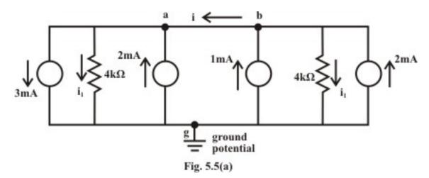
KCL at node 'b':  $i+i_1=2+1=3$  (5.14) KCL at node 'a':  $i+2=3+i_1 \rightarrow i-i_1=1$  (5.15) From equations (5.14)-(5.15), one can get i=2mA (current flows from 'b' to 'a') and  $i_1=1mA$ .
