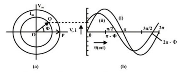
Fig. 13.2 (a) Phasor representation of a sinusoidal (i) voltage and (ii) current, and (b) Waveforms
