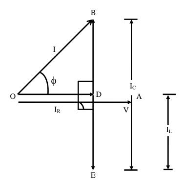
Capacitive (I<sub>L</sub> < I<sub>C</sub>) Fig. 15.4 (c) Phasor diagram
