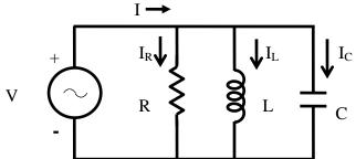
Fig. 15.4 (a) Circuit diagram.
