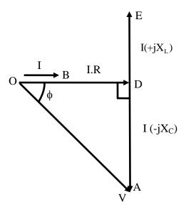
Capacitive (X<sub>L</sub> < X<sub>C</sub>) Fig 15.1 (c) Phasor diagram
